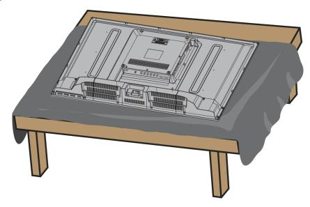
2 Attach the wall-mount bracket to your TV using the mounting holes on the back of your TV. See the instructions that came with the wall-mount bracket for information about how to correctly hang your TV.
